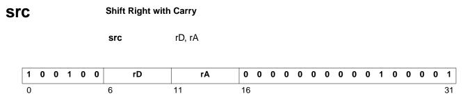
Shifts the contents of register rA, one bit to the right, and places the result in rD. The Carry flag is shifted in the shift chain and placed in the most significant bit of rD. The least significant bit coming out of the shift chain is placed in the Carry flag.
